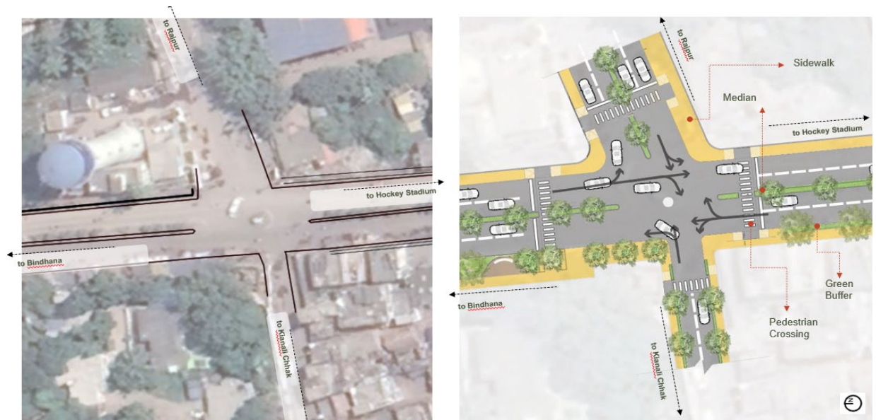
Figure 10: Existing (Left) & Proposed (Right) safe intersection design for Gandhi Chhak Source: UN-Habitat
