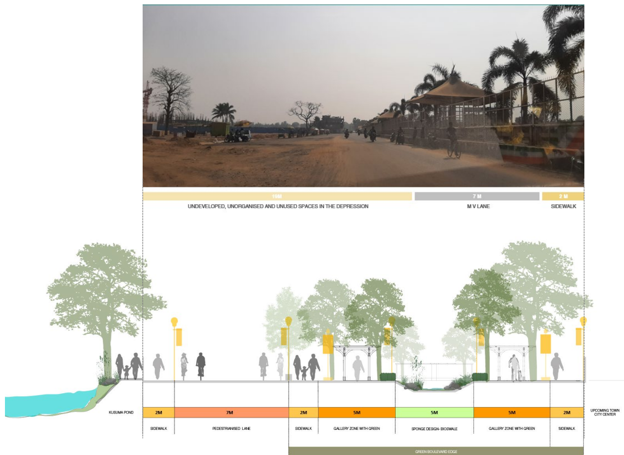
Figure 9: Existing (Above) & Proposed (Below) Street Section for A'-B: Municipal Library – Medical Chhak Source: UN-Habitat
