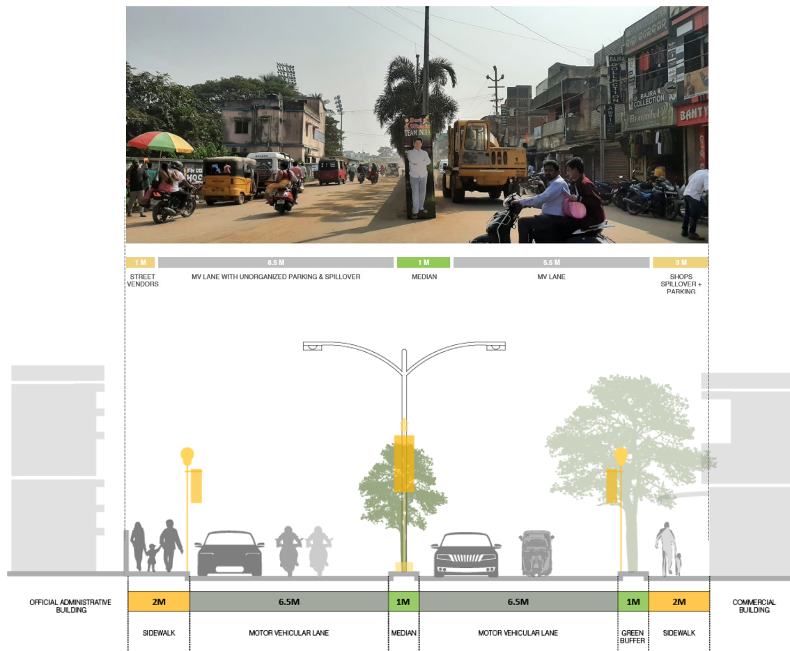
Figure 7: Existing (Above) & Proposed (Below) Street Section for A'-B': Municipal Library – Medical Chhak Source: UN-Habitat
