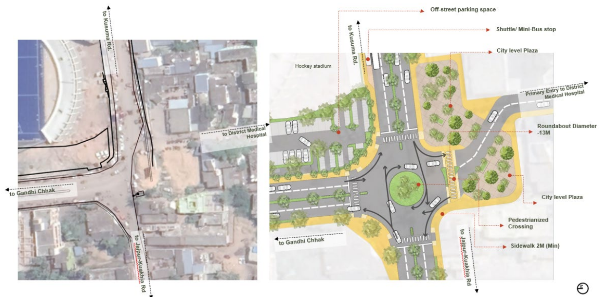
Figure 11: Existing (Left) & Proposed (Right) safe intersection design for Medical Chhak Source: UN-Habitat
