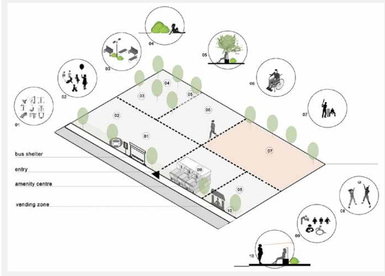
Schematic diagram illustrating activities and design conditions for gender-inclusive public open spaces
