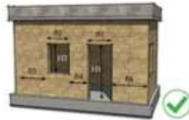
- Openings well away from the corners
