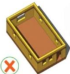
- Too high walls - Long unsupported walls
