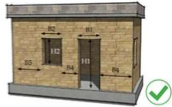
- Openings well away from the corners
