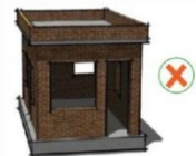
- Too many unreinforced openings (minimum distance between unreinforced openings should be 600mm)
