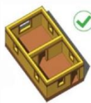
- Wall length < 8 times the thickness - Addition of a buttress wall reduces L/H Ratio
