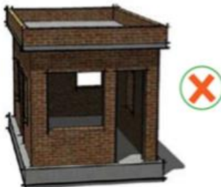
- Too many unreinforced openings (minimum distance between unreinforced openings should be 600mm)
