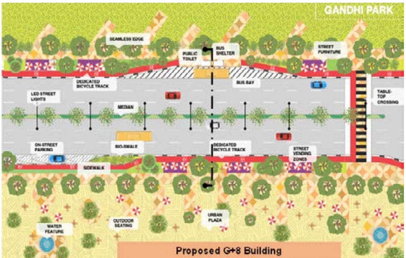
FIGURE 3.12 Proposed cross section of the road with various street elements
